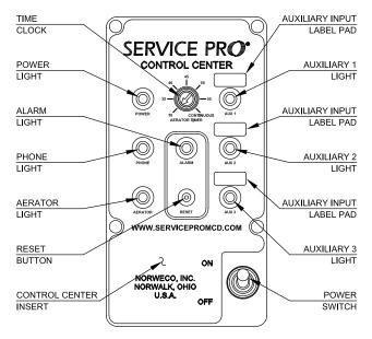
report the specific condition to the Service Pro monitoring center. In the event that any of the auxiliary inputs detect abnormal operation of the treatment system auxiliary equipment, the audible and visual alarms shall immediately activate and the telemetry system shall report the alarm condition to the monitoring center. The service provider shall automatically be notified by the Service Pro monitoring center of the specific alarm condition using phone, fax or email.
